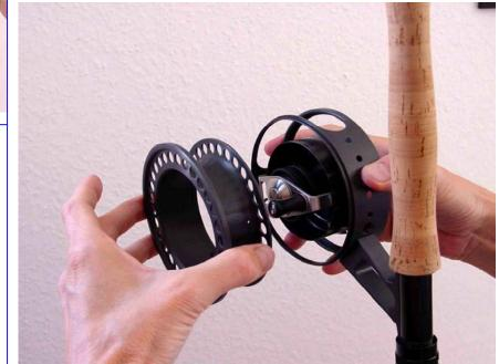
To reinstall the spool, put the spool back onto the reel being careful to align the catches on the reel with the notches on the spool.
