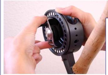
Put the spool back onto the reel being careful not to cant the spool and force it onto the reel.
